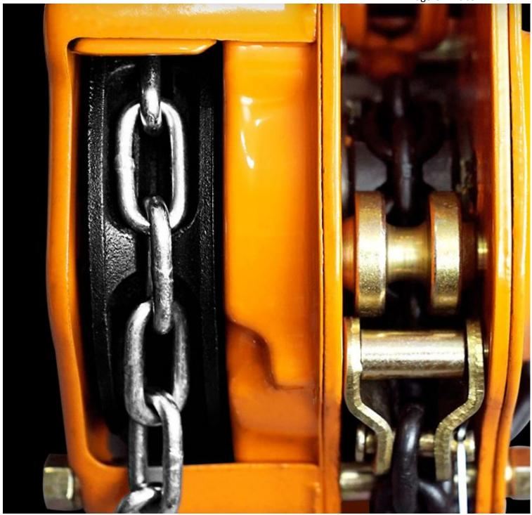
Chain Block2 Ton adopts thickened inner shell, steel bowl with ball bearing, thickened embossed wall board, quenching heat treatment. Flexible and long service life.
